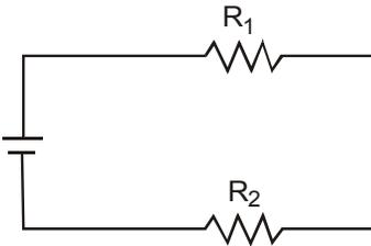
b) Pela Lei de Ohm a corrente é  $i = 12 \text{ Volts} / (2,0 \text{ ohms} + 4,0 \text{ ohms}) = 12 \text{ Volts} / 6,0 \text{ ohms} = 2,0 \text{ A}$  .
